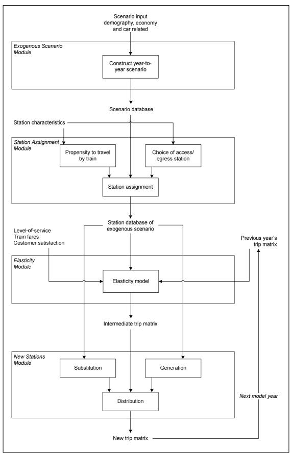
Figure 4. Structure of the Exogenous submodel
