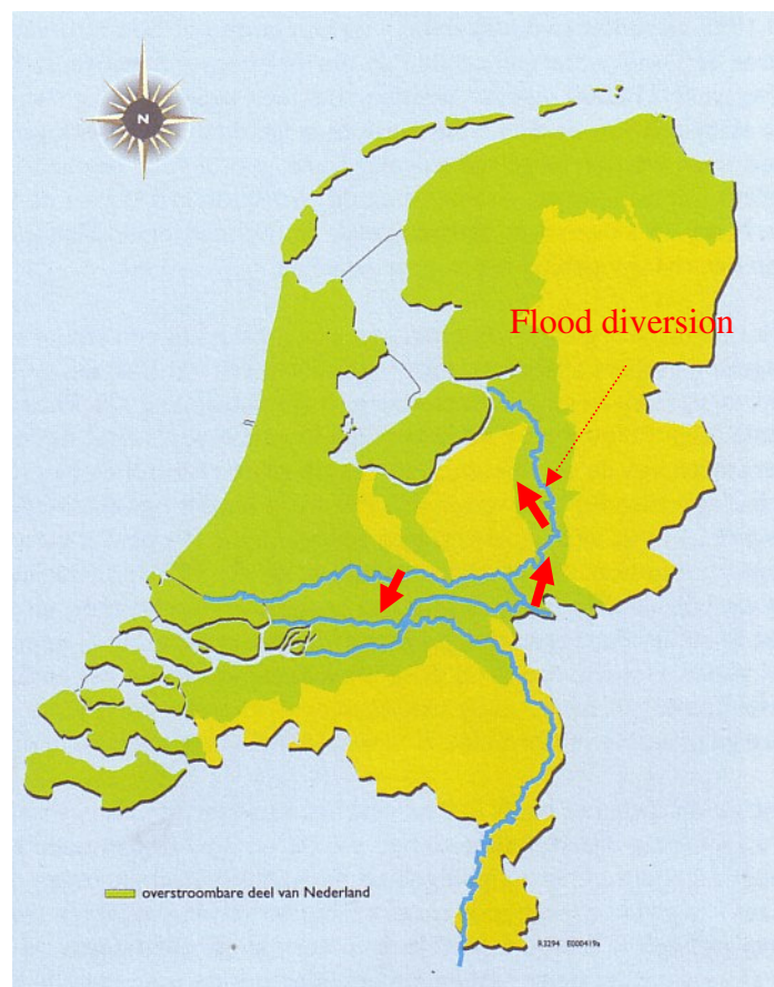
Figure 4: Flood prone areas in The Netherlands – options for flood diversion
